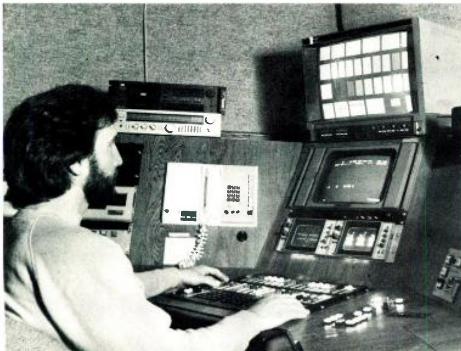
Editel's James Gray checks the setup of a Rank Cintel telecine with TAF. Top monitor shows a positive image of the negative TAF.
